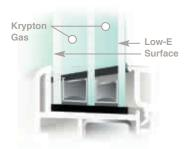
Windows are roughly 80% glass, so it's essential to choose a glass package that delivers superior protection year-round - blocking heat from escaping in the winter and keeping cool air in during the summer. High-performance insulated glass helps ensure a more balanced, comfortable climate with reduced annual fuel costs.
